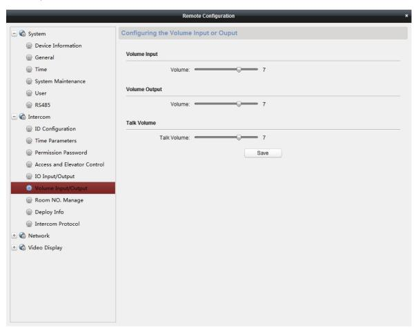
2) After the configuration is completed, the volume of the call between the door station and the indoor station depends on the call volume. The volume of local operation of the door station depends on the touch sound, and the default size is 7.
